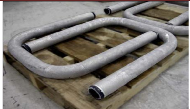
Figure 2: Infiltration brazed 70% tungsten carbide coating applied to the high erosion areas of superheater tube bends
